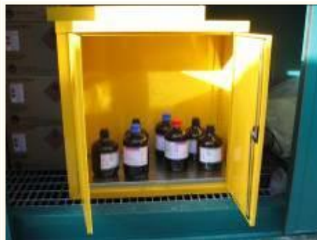
Flammable substances inside the safety cabinet
