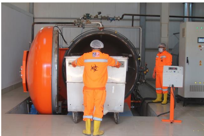
(ZoomPak operational staff preparing the waste for autoclaving)
