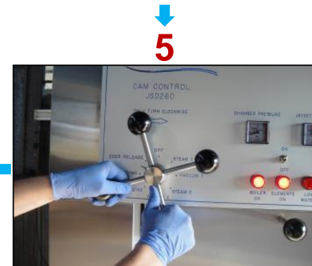
Start heating, multi-vacuum and sterilization cycles
