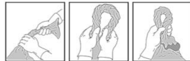
Seal bag when filled to the warning line.
