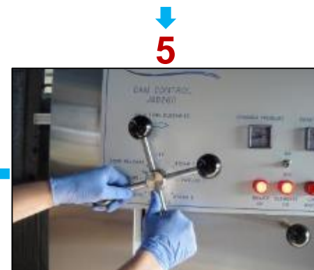
Start heating, multi-vacuum and sterilization cycles
