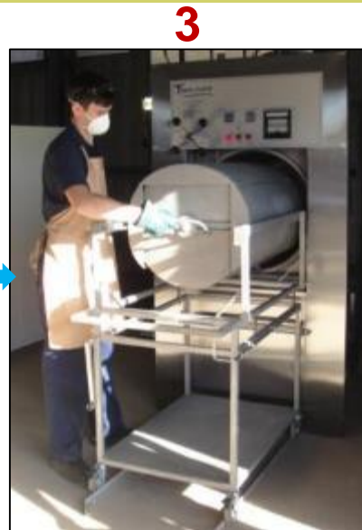
Slide barrel into autoclave
