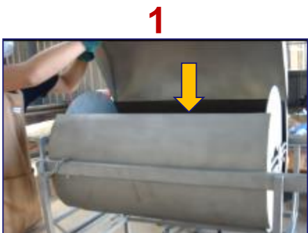
Place waste inside stainless steel barrel and close the lid
