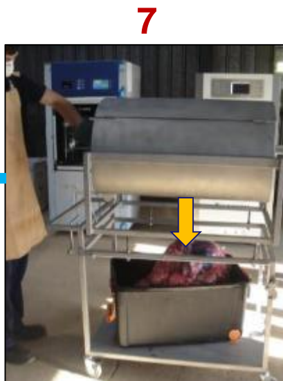
Unlock & rotate barrel to dump treated waste at the bottom
