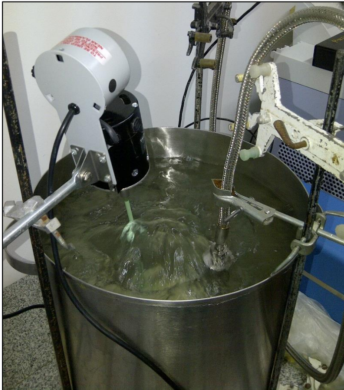
Testing of the reaction vessel (shown without cover), stirrer and ultrasonic probe
